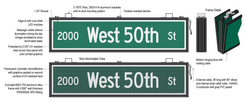
Outdoor full face signs with an aluminum cabinet, edge-lit with cool white LED modules. The sign message is formed by a translucent printed face with a prismatic retroreflective sheeting applied that illuminates when activated and remains viewable when deactivated
