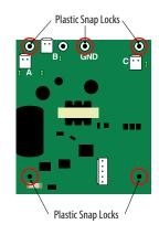
**4.** Place the sign face down on a clean protective surface to avoid scratching the face. Locate the five (5) black plastic snap locks (Christmas trees) holding the power supply to the circuit board. Use needle nose pliers or your fingernail to squeeze the top of the snap lock and pull up on the power supply. Continue around the power supply until it is removed.
