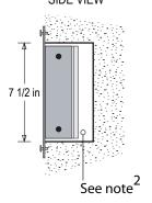
Note<sup>2</sup>: Allow clearance behind sign per local code or per electrical fittings.
